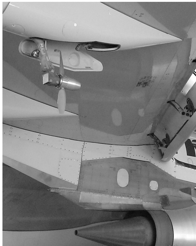
FIGURE 7.5.8 Ram Air Turbine.
