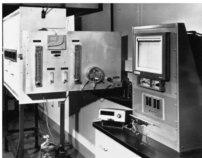
FIGURE 4.1(a) Flooring Radiant Panel Test Apparatus.
