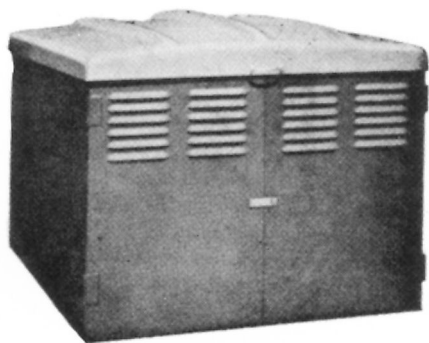
FIGURE A.3.3.18(b) Steel Hose House of Compact Dimensions for Installation over Private Hydrant. House is shown closed; top lifts up, and doors on front side open for complete accessibility.
