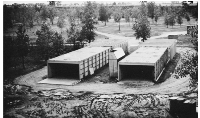
FIGURE 4-1.4(a) Overall view of 20 ft × 100 ft (6.1 m × 30.5 m) fire test building from exhaust end.
