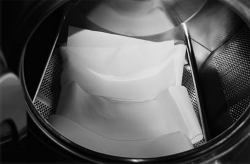
N FIGURE 12.9.3.7(d) Placement of Panel A into Washer/Extractor Drum.
