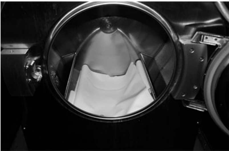
N FIGURE 12.9.3.7(c) Placement of Panel C into Washer/Extractor Drum.
