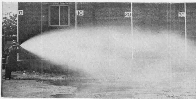
A11.30. A spray nozzle discharge showing the pattern of the spray. Numbers on wall indicate distance from nozzle in feet.
