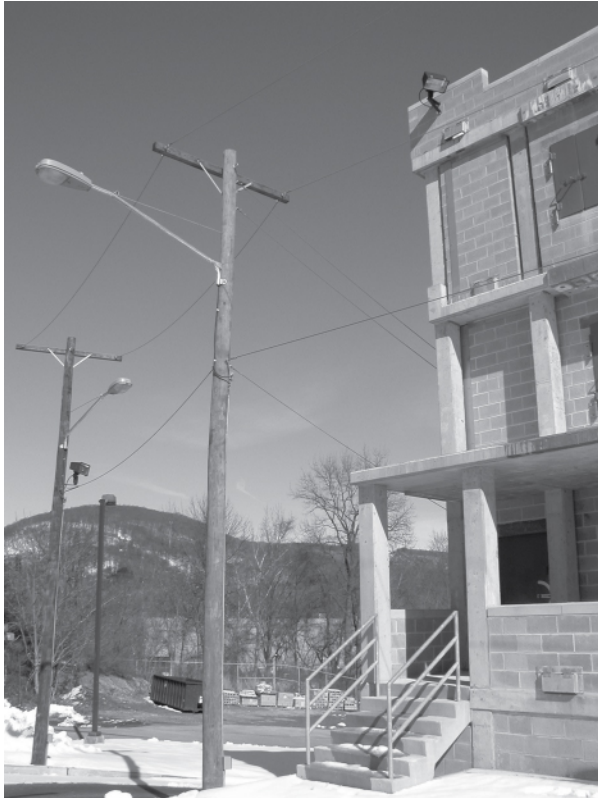
FIGURE B.5.1.4 Simulated Overhead Power Lines Near Training Structure for Laddering Skills. (Courtesy of Reading-Berks Fire Training Center, Berks County, PA)
