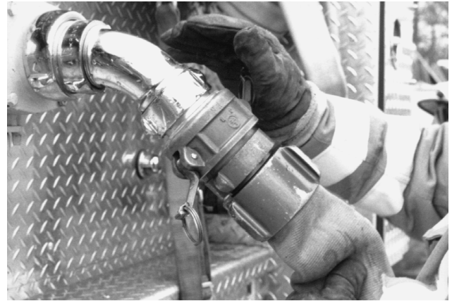
Figure C-1.11 Example of a quick coupling that can help to reduce the fill time.
