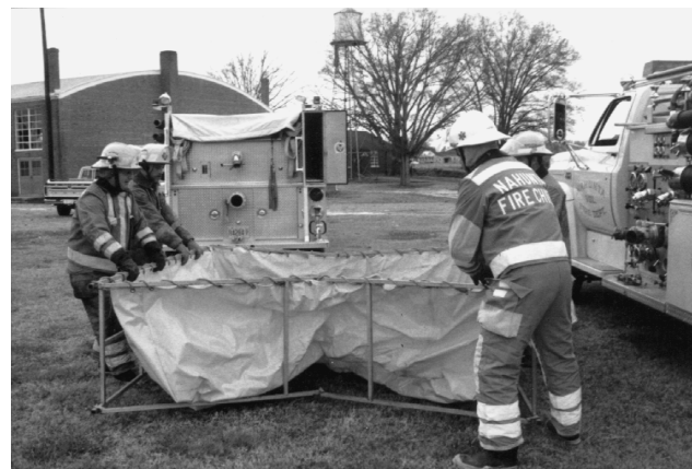
Figure C-1.13(a) Fire fighters set up portable drop tank. (Courtesy of Nahunta Volunteer Fire Department, NC)
