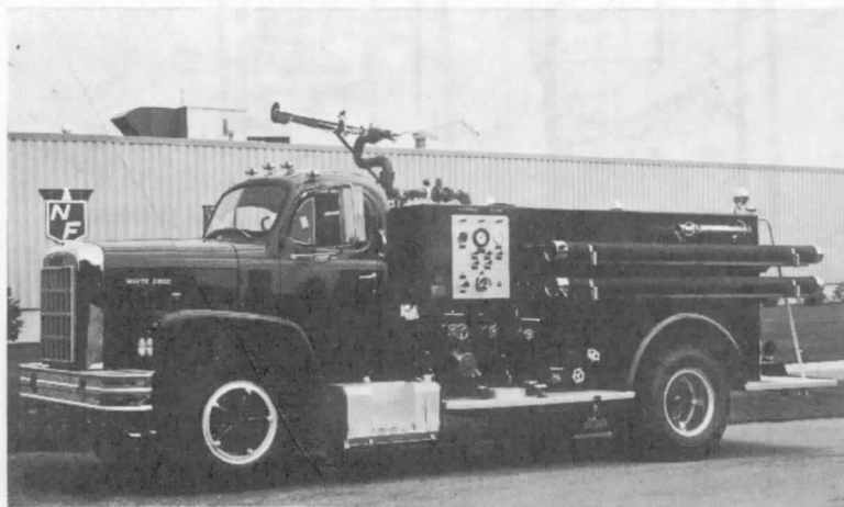
Fig. A-302(f)(1)(a). Standard foam truck-waterpump, proportioning system, airfoam concentrate tank and monitor nozzle.
