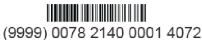
Figure 10 — UHF Gen 2 GS1-128 supplemental backup example, omitting CRC-16
