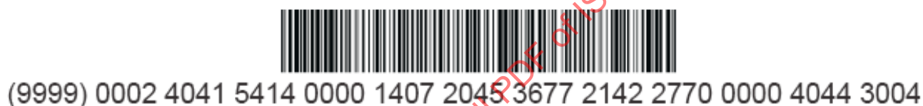
Figure 8 — UHF Gen 2 GS1-128 full backup bar code with octal HRI
