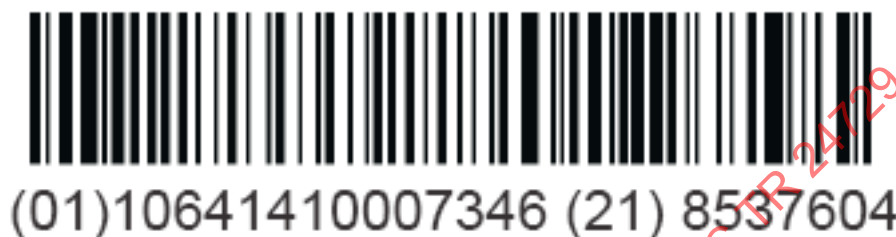
Figure 11 — Partial backup symbol encoding the tag SGTIN data using AIs (01)(21)
