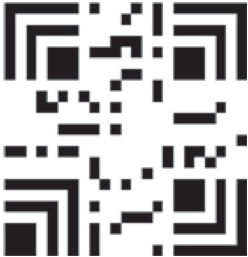
Figure K.4 — Masking result for Figure K.3 with masking pattern 00
