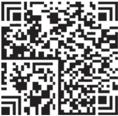
Figure K.15 — Masking result for Figure K.11 with masking pattern 11
