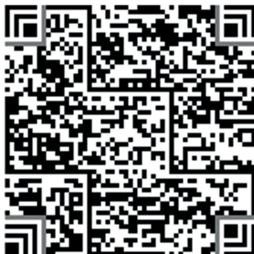
Figure K.18 — Han Xin Code symbol Version 17 after data placement ( K.2 )
