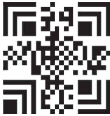
Figure K.5 — Masking result for Figure K.3 with masking pattern 01
