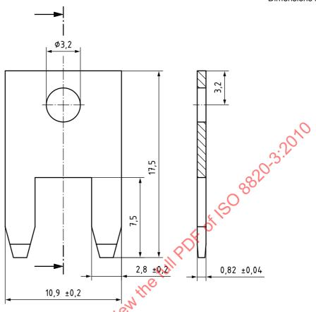
Where not specified in the figure, the common tolerances shall be in accordance with tolerance class m as specified in ISO 2768-1.
