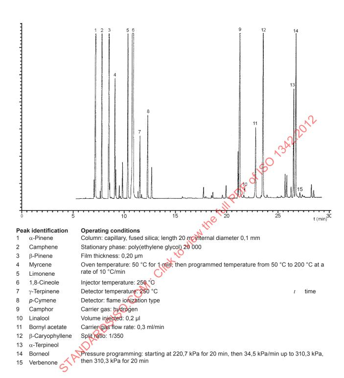
Figure A.2 — Typical chromatogram taken on a polar column for Tunisian and Moroccan type
