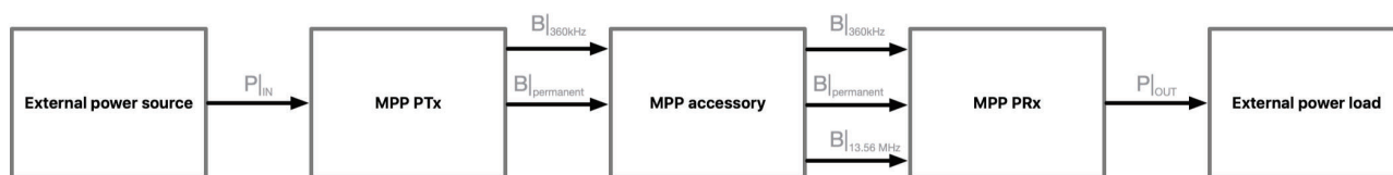
Figure 2.2.2: 3 System block diagram.
