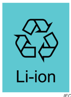
Figure 9 – Example of marking with recycling symbol for lithium ion batteries
