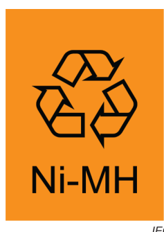
Figure 8 – Example of marking with recycling symbol for nickel metal hydride batteries
