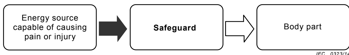
Figure 2 – Three block model for safety
