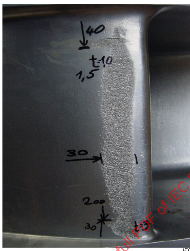
Figure 15 – Leading edge cavitation erosion on a Francis pump-turbine caused by extended periods of operation at very low loads
