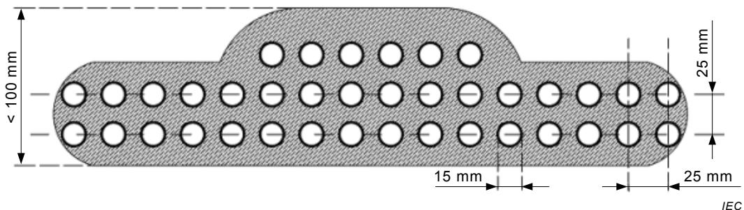
No part of any plate is to project outside of the **heated area**.
