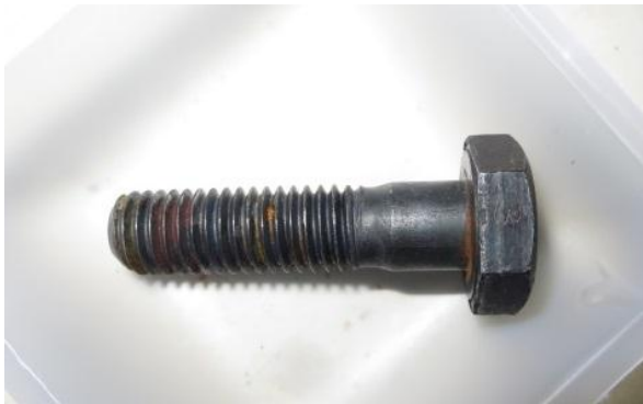
Bolt 3 after deposit removal (0°)
