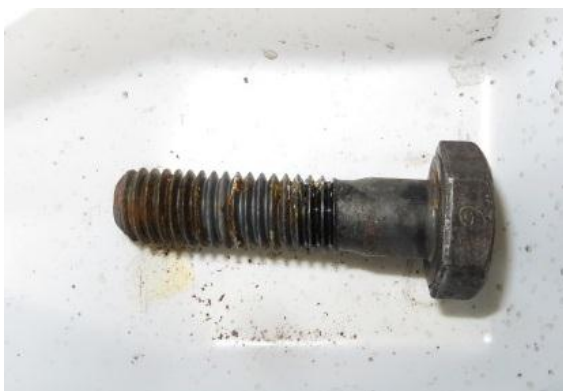
Bolt 6 after deposit removal (0°)
