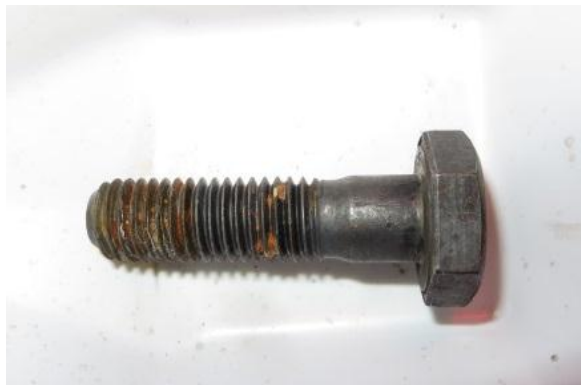
Bolt 4 after deposit removal (0°)
