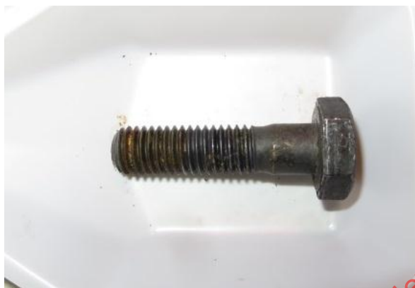
Bolt 2 after deposit removal (0°)
