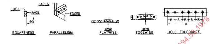
Table 1 Dimensional Tolerances in Inches of Solid Steel Rectangular Metal Cutting Squaring Shear Knives (Dimensions in Inches)
